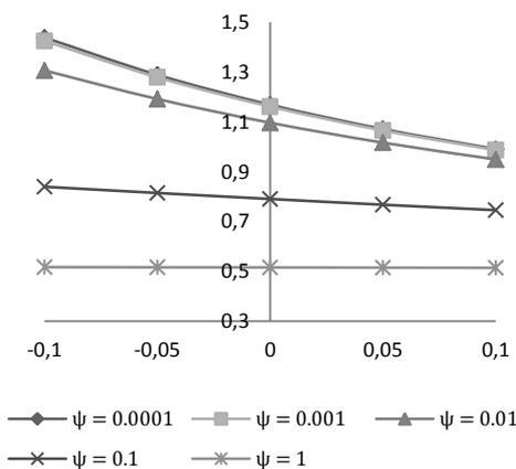
**Fig. 12.** Variation of Load carrying capacity with respect to  $\bar{\alpha}$  and  $\psi$
