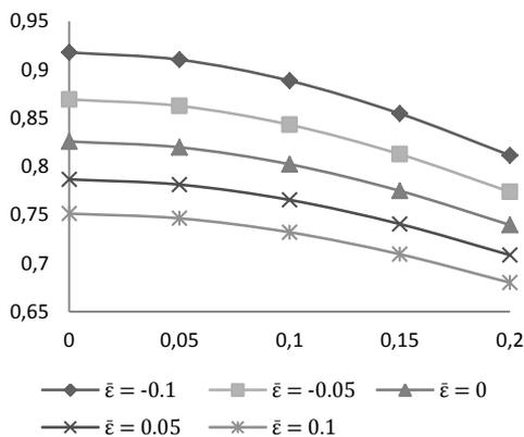
Fig. 7. Variation of Load carrying capacity with respect to  $\bar{\sigma}$  and  $\bar{\varepsilon}$
