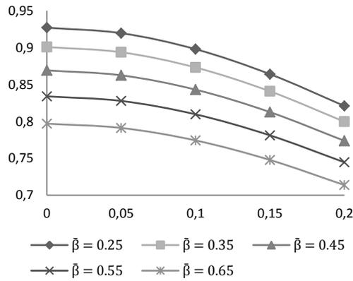
Fig. 8. Variation of Load carrying capacity with respect to  $\bar{\sigma}$  and  $\bar{\beta}$
