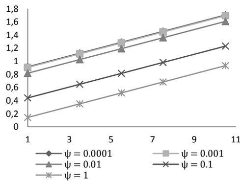
Fig. 5. Variation of Load carrying capacity with respect to  $\mu^*$  and  $\psi$
