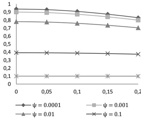
Fig. 9. Variation of Load carrying capacity with respect to  $\bar{\sigma}$  and  $\psi$
