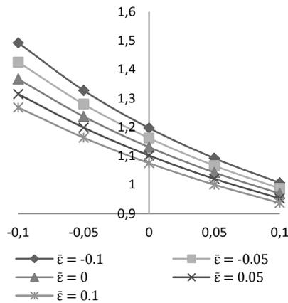
Fig. 10. Variation of Load carrying capacity with respect to  $\bar{\alpha}$  and  $\bar{\epsilon}$
