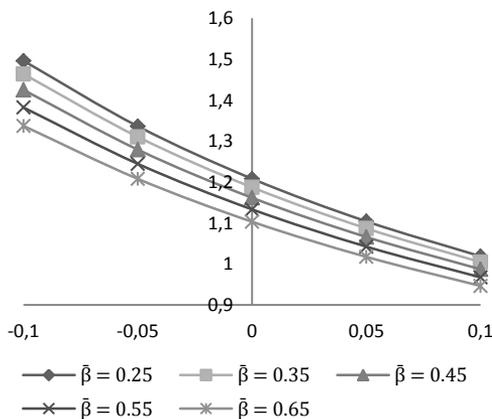
**Fig. 11.** Variation of Load carrying capacity with respect to  $\bar{\alpha}$  and  $\bar{\beta}$
