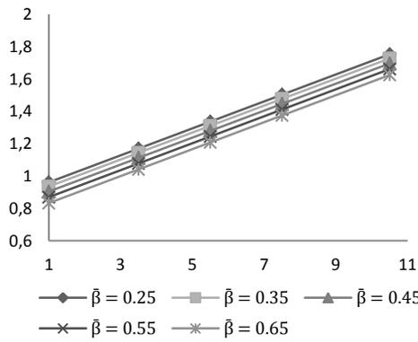
Fig. 4. Variation of Load carrying capacity with respect to  $\mu^*$  and  $\bar{\beta}$
