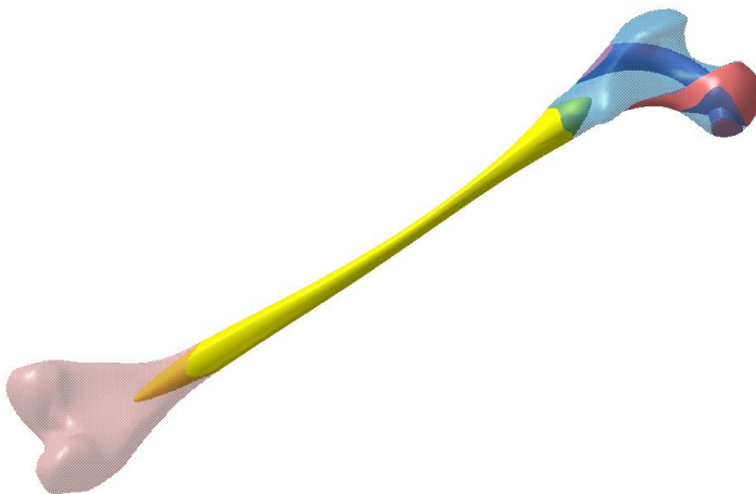
Fig. 3. Zones created inside CAD model of femur, which are then used in FE model creation. The surrounding zone corresponding to cortical bone is hidden in this Figure
