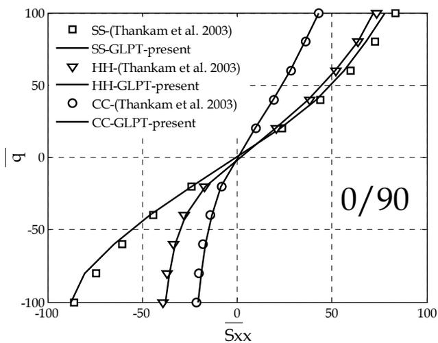
**Fig. 6.** Nonlinear bending of square cross ply 0/90 plate with different boundary conditions and  $a/h = 10$  ; in plane stress  $\bar{S}_{xx}$  versus load parameter.
