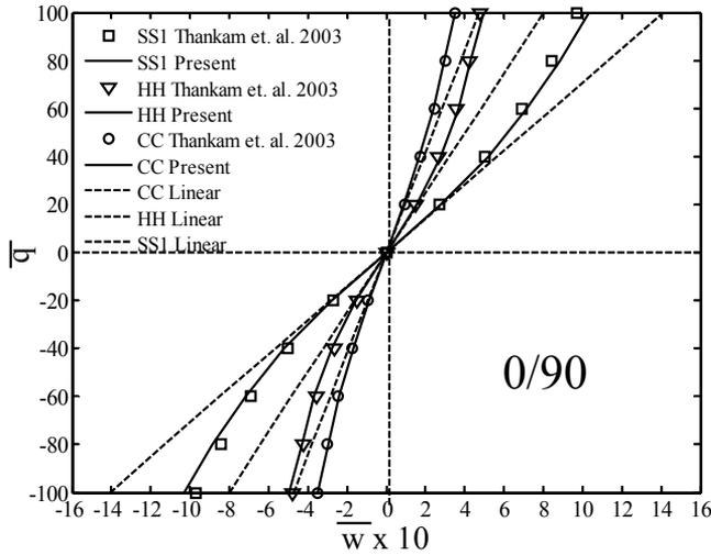
**Fig. 4.** Nonlinear bending of square cross ply 0/90 plate with different boundary conditions and  $a/h = 10$ ; central displacement versus load parameter.
