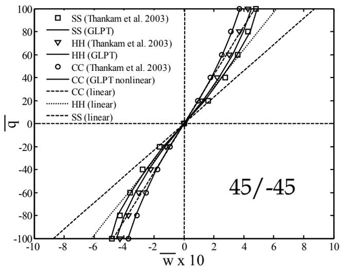
**Fig. 5.** Nonlinear bending of square angle ply 45/-45 plate with different boundary conditions and  $a/h = 10$  ; central displacement versus load parameter.
