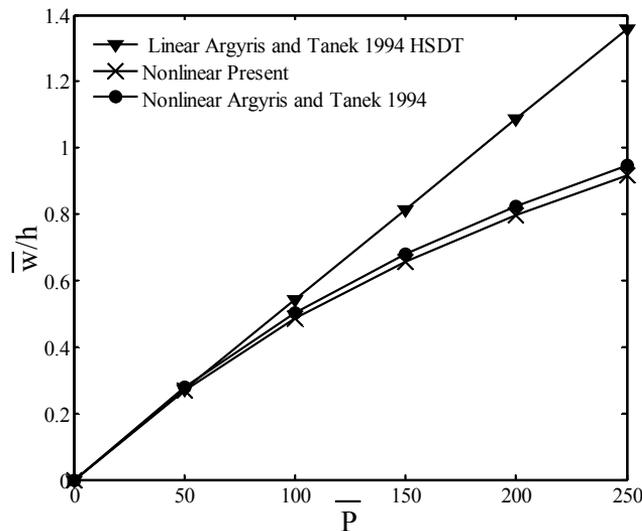
**Fig. 8.** Nonlinear bending of square simply supported (SS1) general quasi-isotropic (0/45/-45/90)s laminated plate with  $a/h = 10$ ; central displacement versus load parameter
