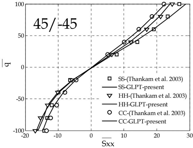
**Fig. 7.** Nonlinear bending of square angle ply 45/-45 plate with different boundary conditions and  $a/h = 10$ ; in plane stress  $\bar{S}_{xx}$  versus load parameter.
