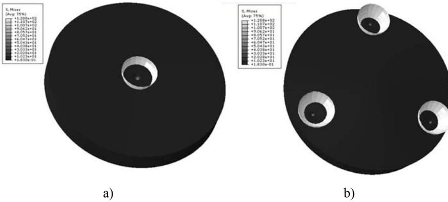
**Fig. 3.** Contours of von Mises stress at a punch displacement ( $D_p$ ) of 0.05 mm for the specimen with a Poisson's ratio ( $\nu=0.35$ ) and elastic modulus ( $E=3000$  MPa): (a) upper view and (b) lower view.
