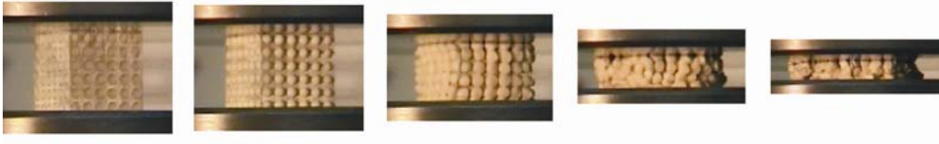
Fig. 3. Compression and collapse of the specimen with the silicone filler.
