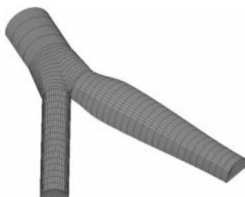
**Fig. 2.** A FE model of the carotid artery bifurcation generated using the parameters shown in Fig. 1.
