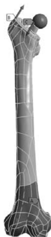
Figure 5. Boundary conditions of the finite element model: A) Lower region, fully fixed, B) Resulting muscle force, C) Femoral head loading.
