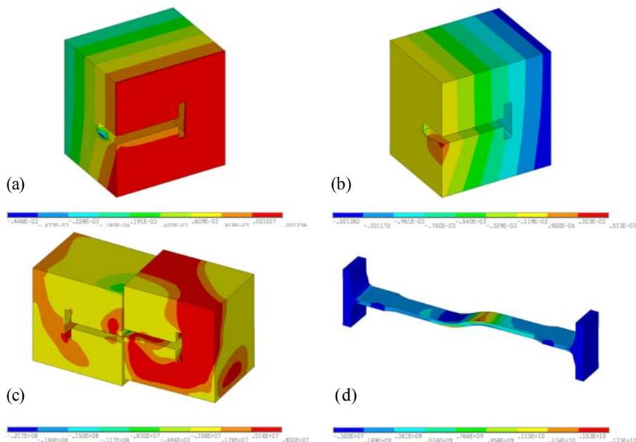
**Fig. 9.** Model R. The distribution of displacements along (a) x-axis [m] and (b) y-axis [m]; (c) the maximum principal stress  $\sigma_1$  [Pa]; (d) the equivalent Mises stress in the connector [Pa].
