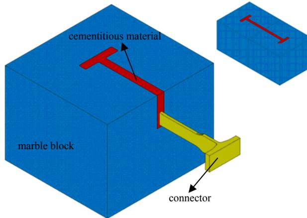
**Fig. 1.** The connection of epistyles by means of "I" shaped connectors.
