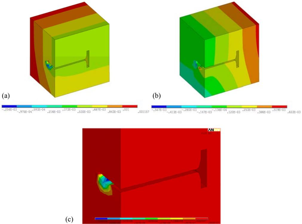
**Fig. 11.** Model NM. The distribution of (a) displacements along x-axis [m]; (b) displacements along y-axis [m]; (c) the maximum principal stress  $\sigma_1$  [Pa].
