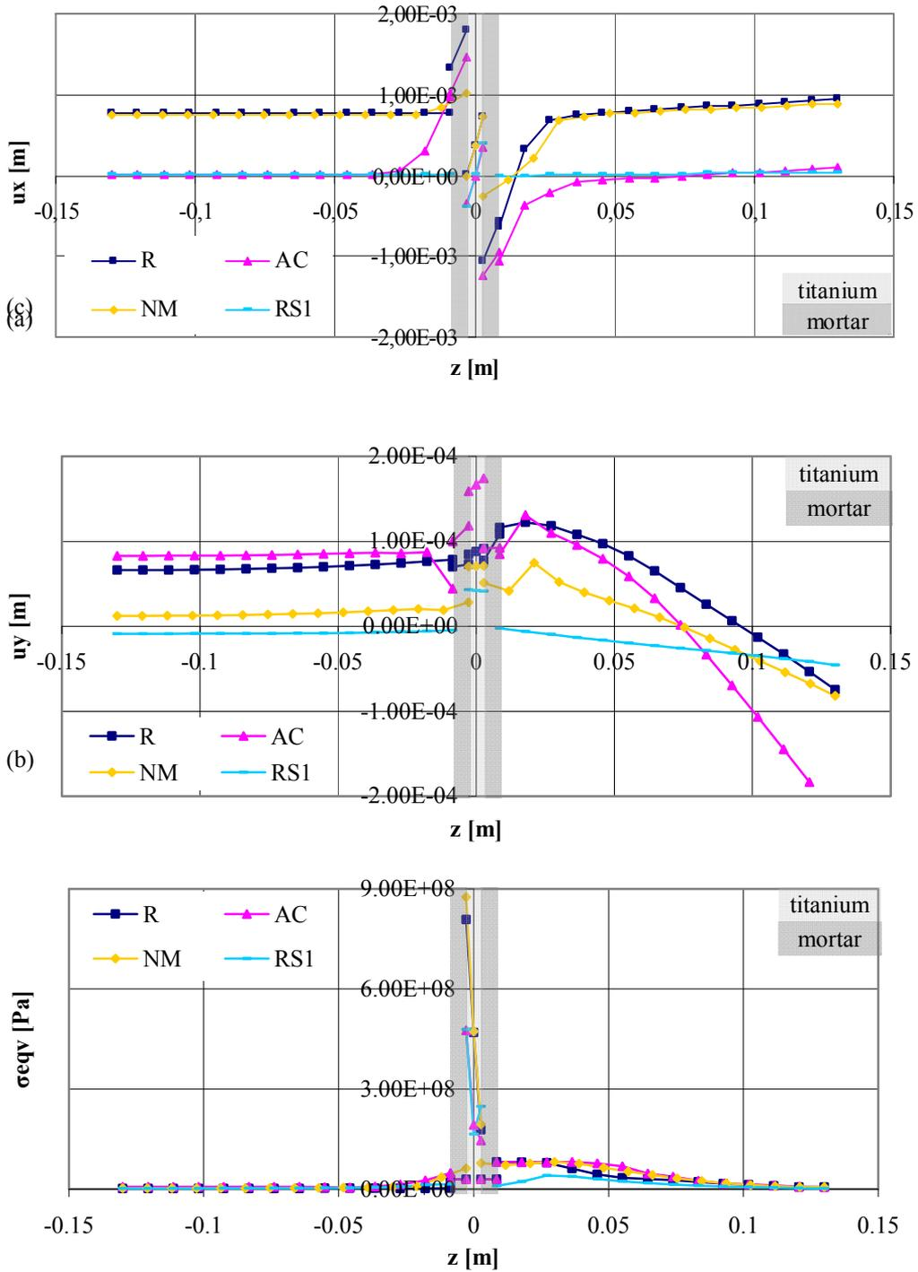
Fig. 14. The variation of the x- (a) and y- (b) components of displacement along the path AA' and the variation of the von Mises equivalent stress (c) along the same path.
