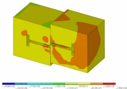
**Fig. 10.** Model AC. The distribution of the maximum principal stress  $\sigma_1$  [Pa].
