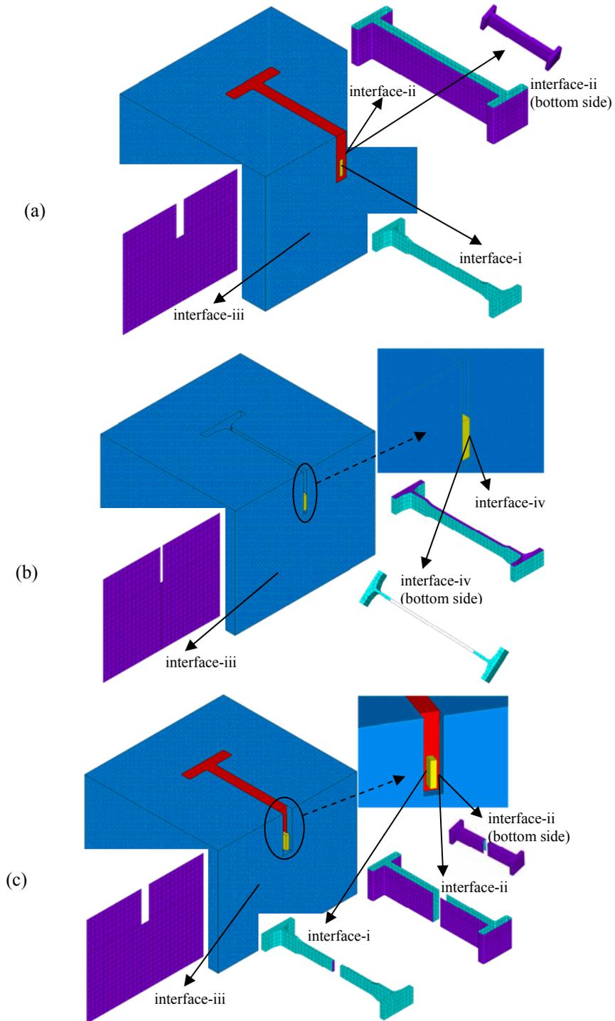
**Fig. 8.** The position and the shape of the material interfaces for (a) Models R and AC; (b) Model NM; (c) Model RS1.
