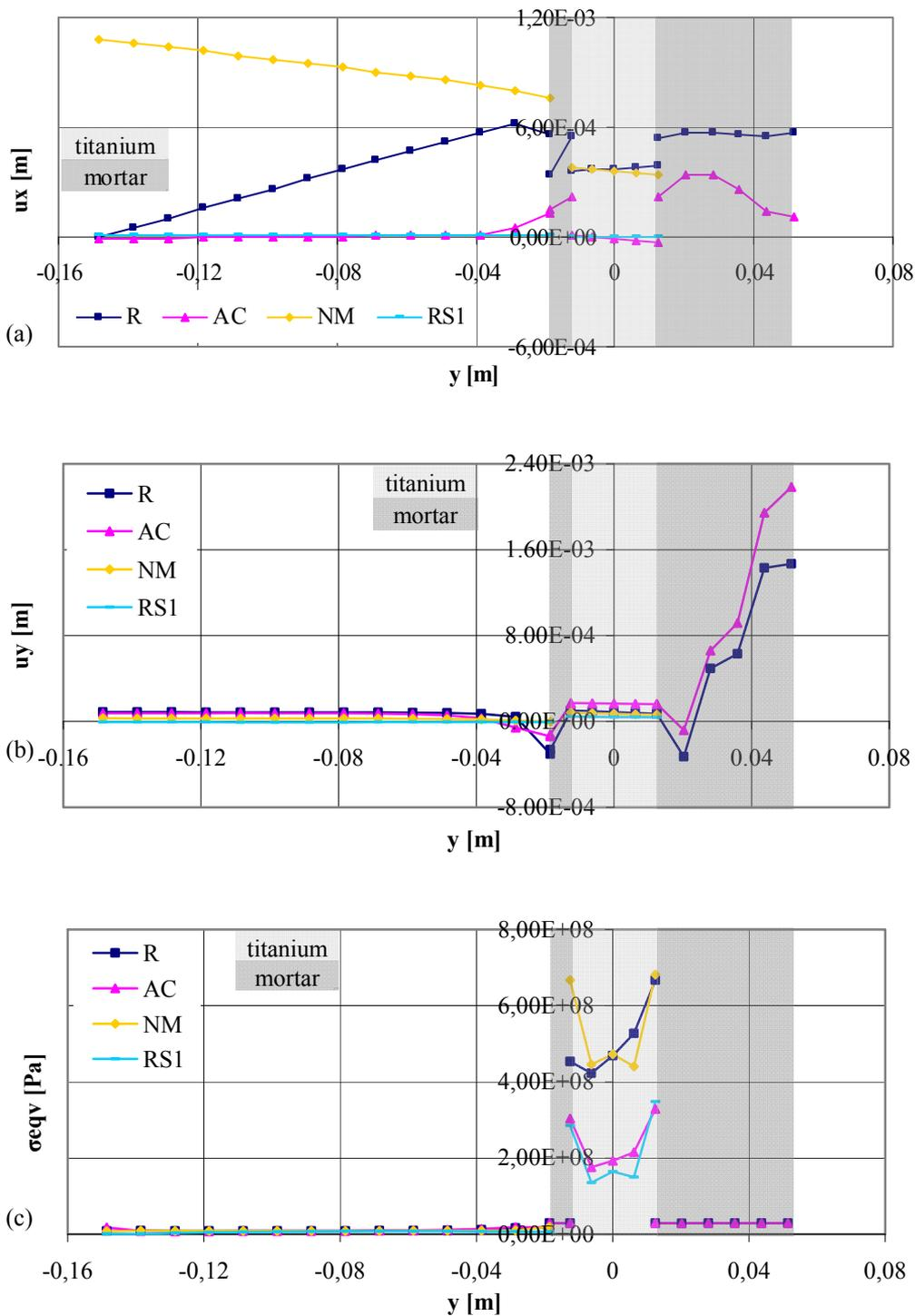
**Fig. 15.** The variation of the x- (a) and y- (b) components of displacement along the path BB' and the variation of the von Mises equivalent stress (c) along the same path.
