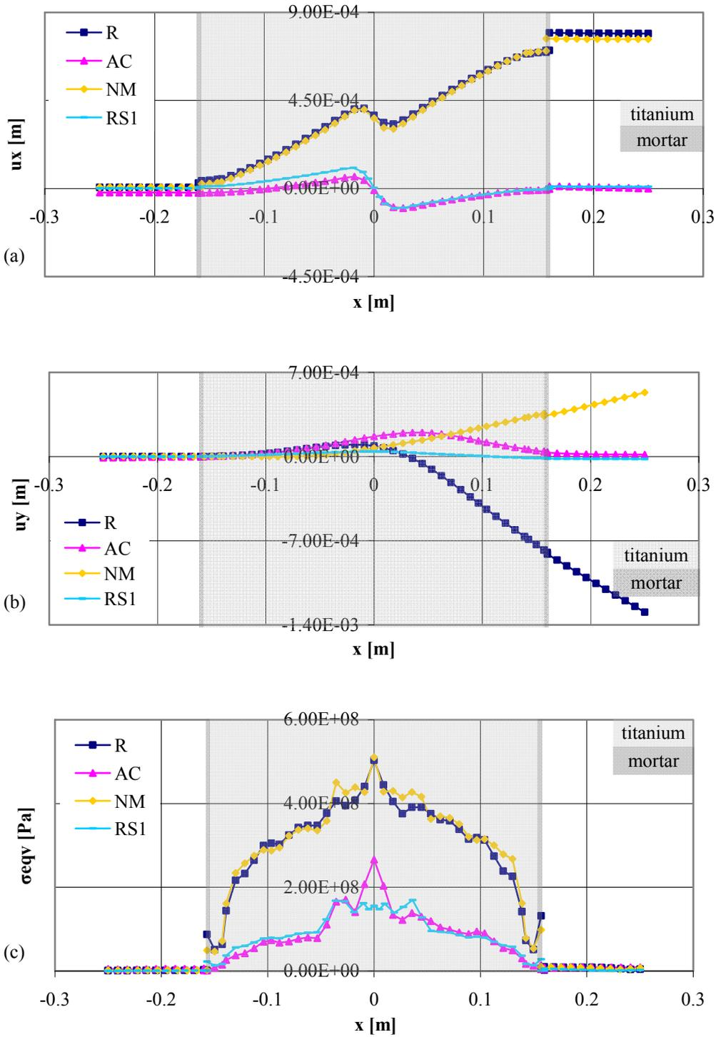
**Fig. 16.** The variation of the x- (a) and y- (b) components of displacement along the path  $CC'$  and the variation of the von Mises equivalent stress (c) along the same path.
