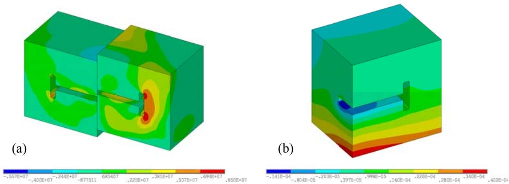
**Fig. 12.** Model RS1. The distribution of (a) the maximum principal stress  $\sigma_1$  [Pa]; (b) displacements along x-axis [m].
