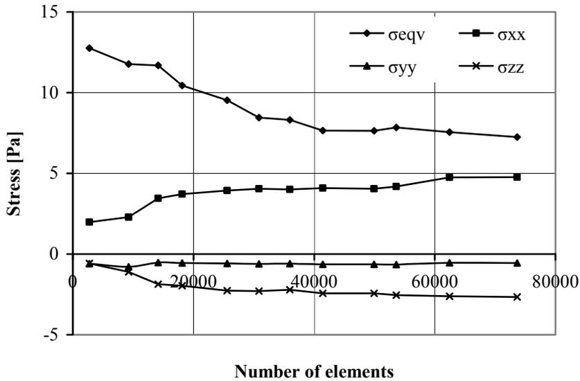
**Fig. 7.** The variation of the stress components at the central point of the central section of the connector vs. the number of elements.
