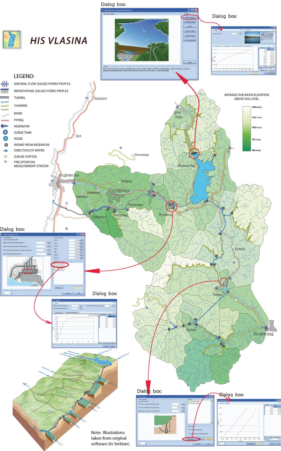
Fig. 4. Illustration of hydro-information system “Vlasina”
