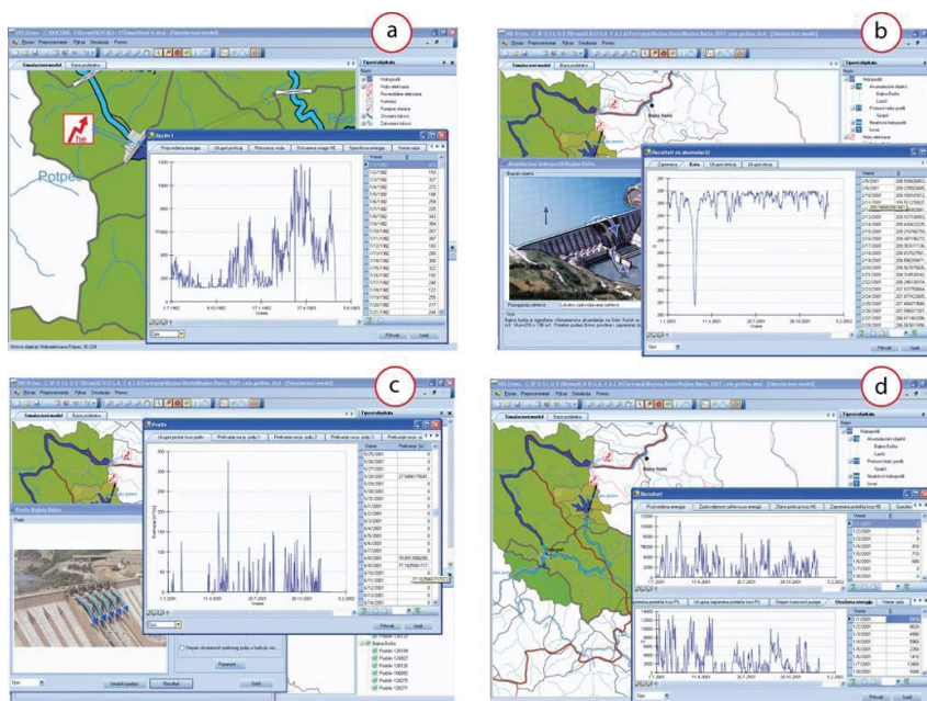
Fig. 13. Simulation Results (a – electricity generation on “Potpeć” HPP, b – realized water level in the “Bajina Bašta” storage, c – water spilling on the “Bajina Bašta” storage and d – reversible power plant operation).
