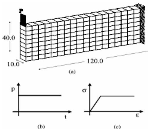
**Fig. 12.** (a) Geometry (in mm) and discretization, (b) loading history and (c) material description.
