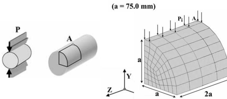
**Fig. 8.** Geometry and discretization of a cylinder-splitting test
