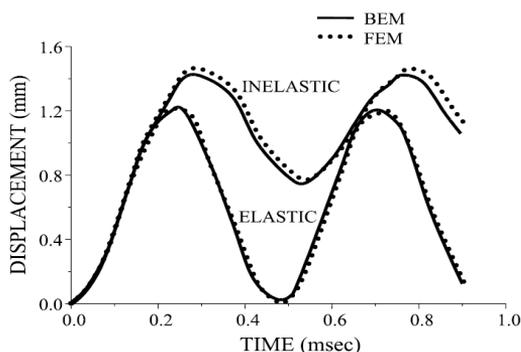
**Fig. 13.** Vertical displacement history at load point.
