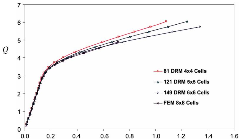
Fig. 5. Center point deflection computed by BEM and FEM.
