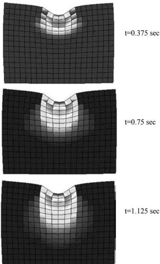
**Fig. 11.** Displacement and inelasticity region on the FEM mesh.
