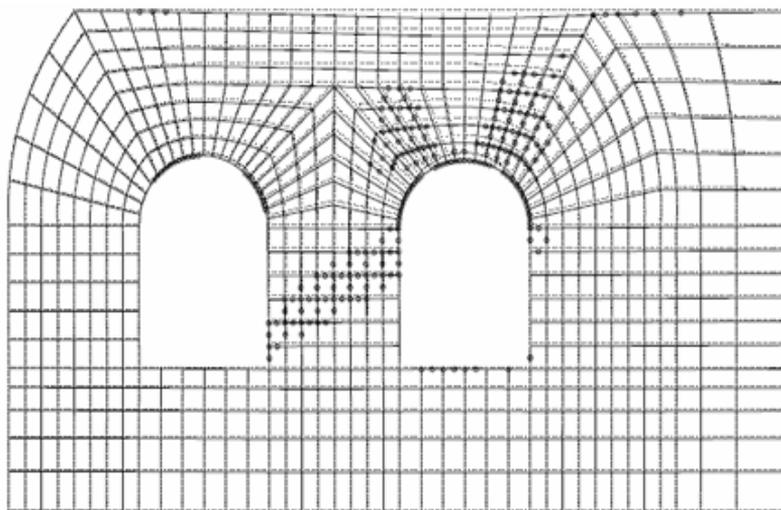
**Fig. 2.** Deformed mesh and yielded nodes.
