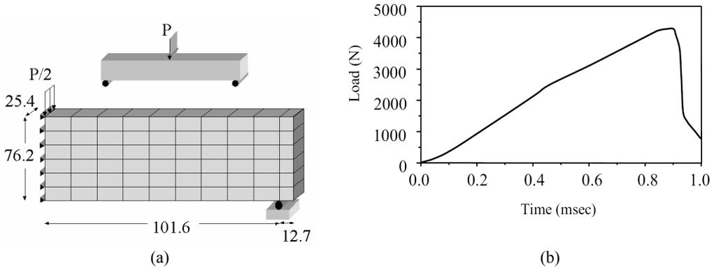
**Fig. 14.** a) Geometry (in mm) and boundary element discretization, b) Loading history.
