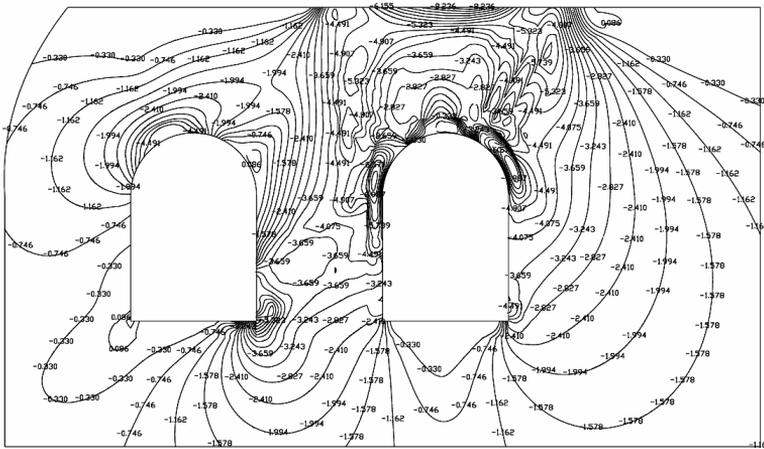
Fig. 3. Compressive stress contours.
