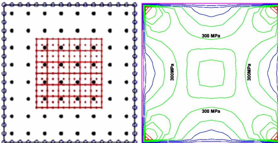
Fig. 4. Typical BEM mesh and iso-stress contours of plastic zones.
