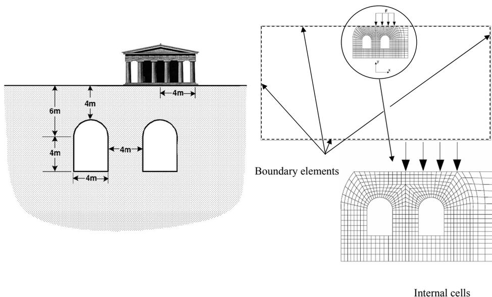
**Fig. 1.** Geometry and BEM discretization of the Example 4.1.
