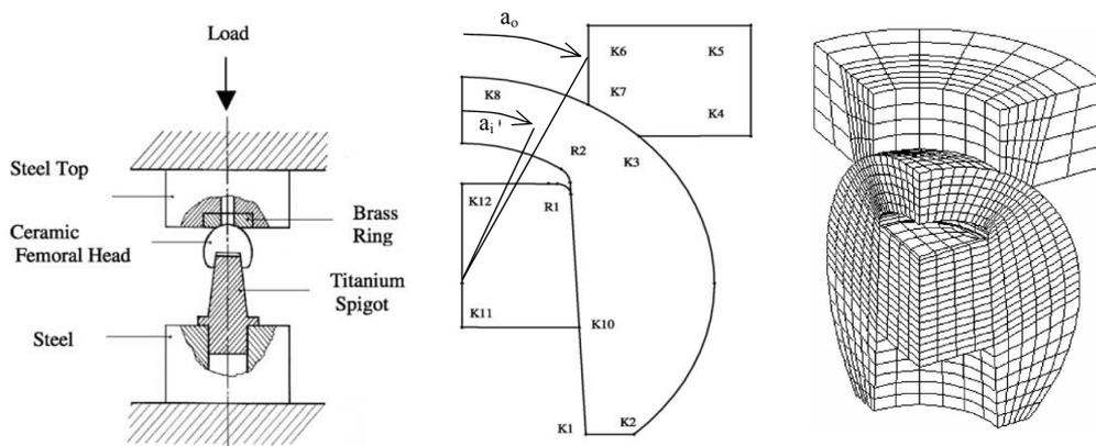
Fig. 6. Physical problem and BE mesh for femoral head assembly.
