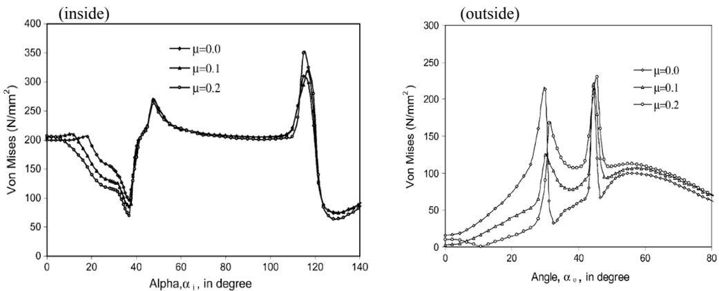
**Fig. 7.** Elasto-plastic stress distribution around the inside and outside of the femoral head.
