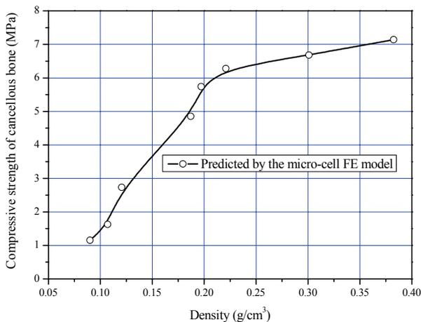
**Fig. 7.** Compressive strength versus density of the interface.
