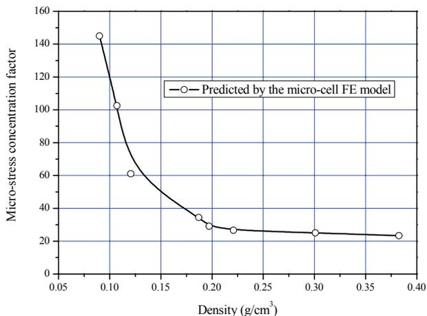
**Fig. 6.** Micro-stress concentration factor in the micro-architecture of cancellous bone.
