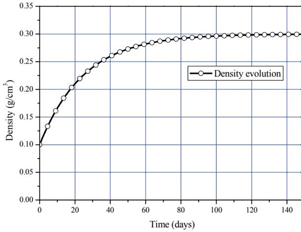
**Fig. 5.** Density evolution of the implant / mandible interface (from unhealed to healed state).
