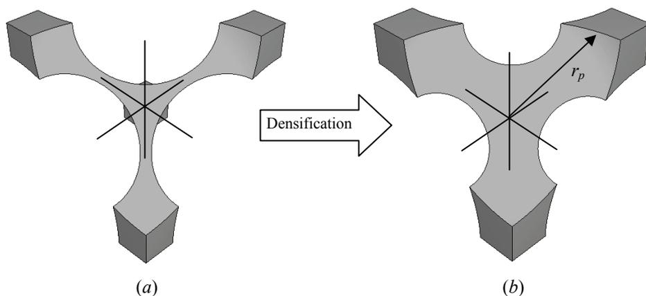
**Fig. 4.** Micro-stress analysis of the micro-architecture of cancellous bone, (a) Unhealed: density of  $0.1 \text{ g/cm}^3$  and (b) Healed: density of  $0.3 \text{ g/cm}^3$ .
