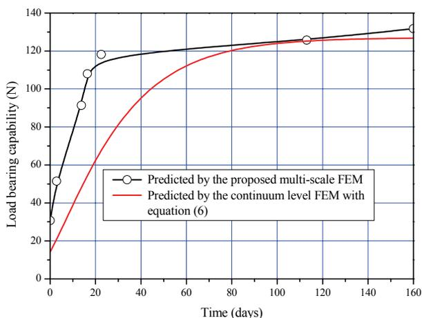
**Fig. 10.** Multi-scale finite element prediction on load bearing capability.
