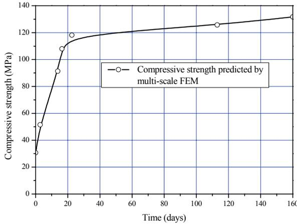
**Fig. 8.** Evolution of compressive strength.
