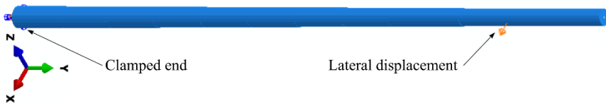
Fig. 7. Geometry of the one-dimensional numerical model, boundary condition and load
