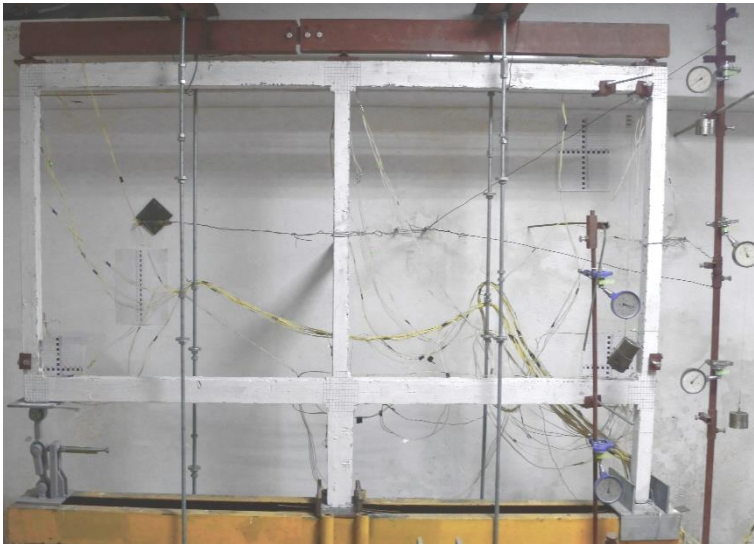
Fig. 4. 2D scale model of RC moment frame investigated by Savin, Kolchunov and Korenkov (2020). (a) Reinforcement scheme; (b) General view of the frame (mirrored to the reinforcement scheme).
