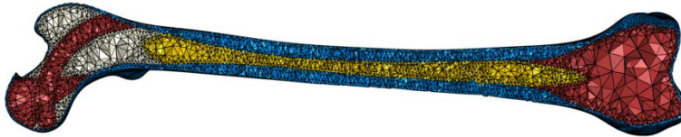
Fig. 19. Finite elements created inside various zones of FEM model. Equivalent moduli of elasticity assigned to each of the zones: compact bone – 17GPa, spongy bone of higher trabecular density – 0.4 GPa, spongy bone of lower trabecular density – 0.1 GPa (Trajanović 2010)
