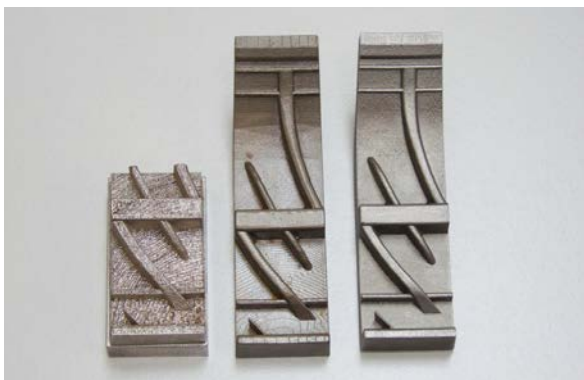
Fig. 30. The one-pitch-segments made by SLM, SLS and DMLS
